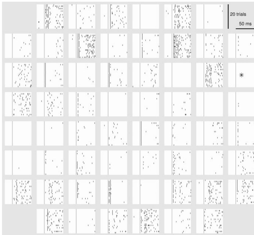
Figure 4. Array-wide responses to stimulation. Each graph shows the responses on one electrode, represented according to the geometry of the array. The stimuli were delivered to the marked electrode. Vertical line indicates time of stimulation. Spikes were detected after artifact suppression (Wagenaar and Potter, 2002); TTX control confirmed the biological origin of all detected spikes.
